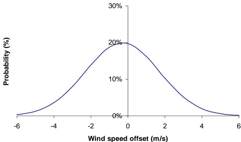
**Figure 7. Example of the probability function for the block-averaged wind speeds for the individual wind turbines in an area at a given time. An offset adjustment of  $-0.15$  m/s results in an unchanged accumulated production for the aggregated multi-turbine power curve and the given wind speed distribution.**
